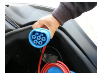
Fig 8 – Type 2 kontakt for Mode 3
